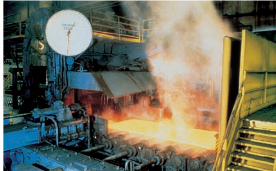
Accurately measuring temperature of slabs, billets, or blooms on a hot rolling mill ensures consistent product quality.
