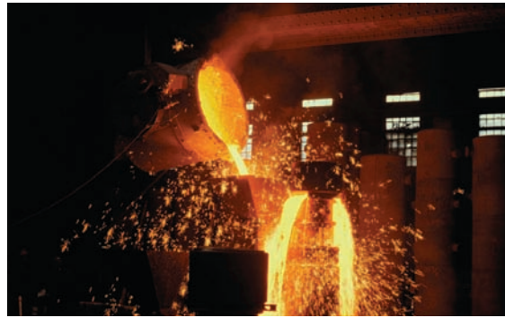
Monitoring temperature of molten metal prior to and during pouring ensures correct metallurgical properties.
